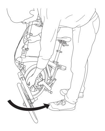
4 Align the front wheel hub cap to be over the rear wheel hub nut.
